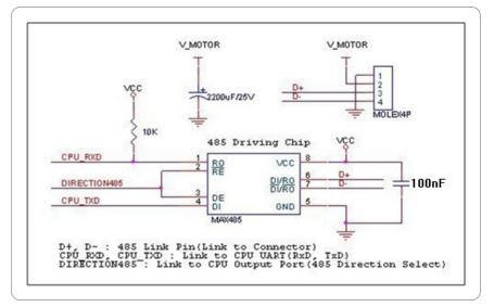
The power of Dynamixel is supplied via Pin1(-), Pin2(+).
