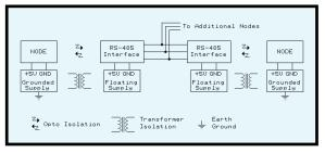
Figure 3—A galvanically isolated link has no ohmic connection to earth ground or to the other circuits the network connects to.
