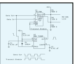
use a hardware or software timer to estimate the time needed to transmit.
